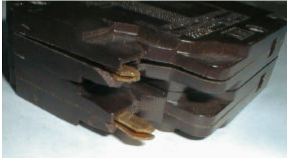
Figure 7 – Damaged “E” type breaker
